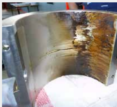
Deposits on bearing material
