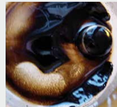
Poor thermal stability Significant deposits
